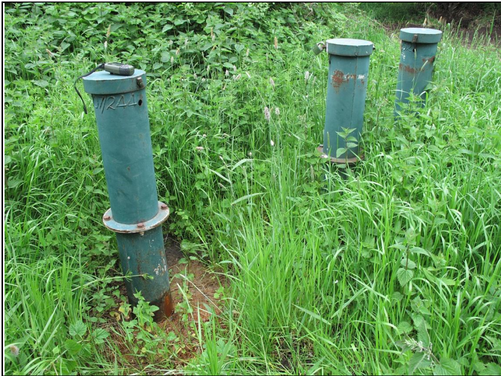
Photo 11: Near to ground level of TM07/244. Water rising in tube and leaking out.
