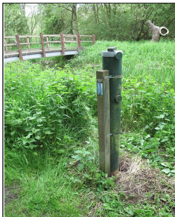
Photos 4 and 5 :TM07/248 Little Ouse Stageboard with automatic recorder, between Old Fen and Blo' Norton Fen.
